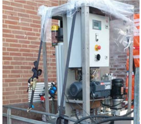
RMF Vacuum Dehydration Units are designated oil purification units that can be applied directly to various types of machine reservoirs. The units dehydrate and clean most types of oil such as lubricating, hydraulic, transformer, and switch oils by removing particles, gasses, and water.
